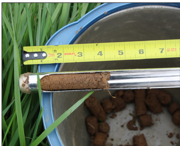
Figure 2. A soil probe should always be used to collect soil samples. Sampling depth for pastures and hayfields should be 4 inches.
